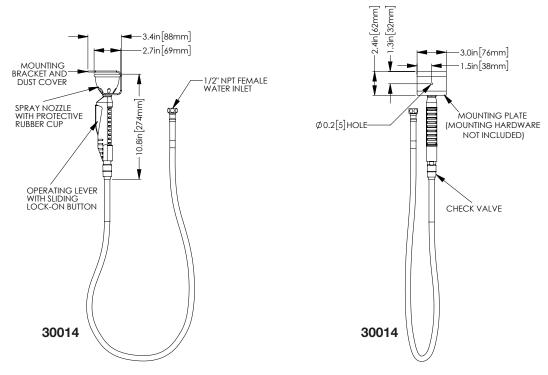
VARIATIONS IN MANUFACTURING AND ASSEMBLY ALLOW FOR ±1/8 in [3 mm] PER THREADED JOINT.
